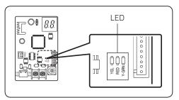
2 When the communication with upper level (e.g.: between DMS and FCU interface module) is detected as valid communication. RED LED will blink.
