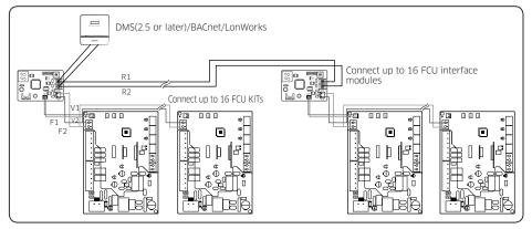
• Maximum number of FCU interface module and FCU KIT that can be installed to a channel of DMS is 16 and 128.
