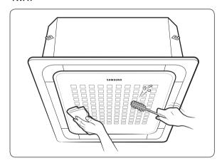
Wipe the surface of the unit with a slightly wet or dry cloth when needed. Wipe off dirt of oddshaped areas by using a soft brush.
