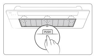
Press the **Push** signs on the front panel, then open the grille.
