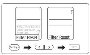
After cleaning and reassembling the air filter, be sure to reset the filter-cleaning reminder as follows:
