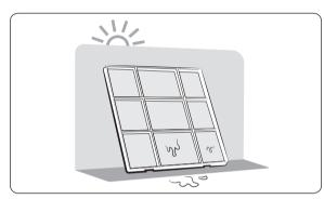
Clean the air filter with a vacuum cleaner or soft brush. If dust is too heavy, then rinse it with running water and dry it in a ventilated area.
