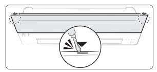
Insert a driver at the marked points and open the front grille.
