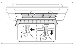
Grab the handle of the air filter and lift it upward while pushing the handle slightly. Pull out the air filter from the indoor unit.
