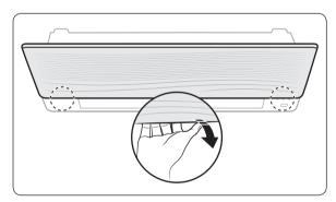
Insert your hand into the front grille and pull out the front grille to open it.
