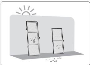
Clean the air filter with a vacuum cleaner or soft brush. If dust is too heavy, then rinse it with running water and dry it in a ventilated area.
