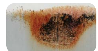
Normal cabinet material after 600 hours
