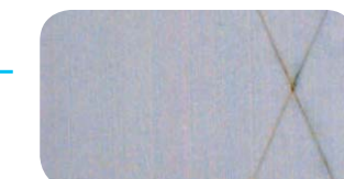
Samsung's rust-free cabinet material after 1000 hours
